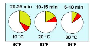
At temperature lower than 10°C (50°F) the hardening can be not homogeneous and even with consequent decrease of the mechanical properties of the hardened adhesive
